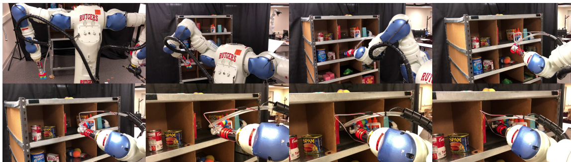
Figure 12. The solution path produced by JIST is executed on the system in an open-loop fashion, and corresponding frames of this execution along with the timestamps are shown here. The Motoman begins executing a motion plan (top left) computed for reaching an object located behind some clutter, ending with a grasp (bottom right).
